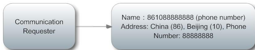
Figure 1 - Addressing Mode NAS (Telecom network)
